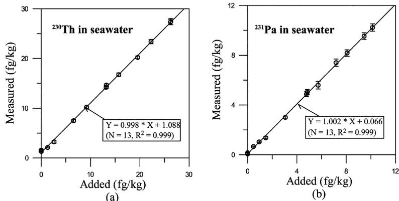
Fig. 3. Standard addition of  $^{230}\text{Th}$  (a) and  $^{231}\text{Pa}$  (b) to coastal waters and linear regression on the data.
