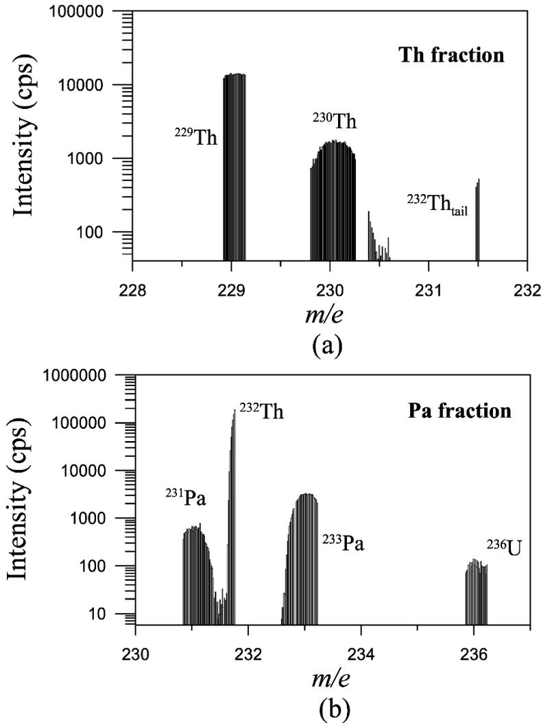
Fig. 1. Sector type ICP/MS spectra for Th (a) and Pa (b) obtained from seawater collected in the eastern Atlantic (St. M) at 1500 m. Concentrations are calculated by selecting only the channels corresponding to the top of the peaks after exporting the raw data into an Excel™ spreadsheet, and subtracting isobaric interferences from the  $^{232}\text{Th}$  tail estimated from the counts measured at mass 231.5 and the count ratios reported in Table 2.
