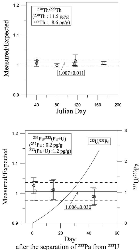
Fig. 2. Variability of isotope ratios measured on monitor solutions produced by combining calibrated Th (11.5 pg/g  $^{230}\text{Th}$  plus 8.6 pg/g  $^{229}\text{Th}$ ) and Pa (0.2 pg/g  $^{231}\text{Pa}$  plus 1.2 pg/g  $^{233}\text{Pa}$ ) standard solutions. The gradual increase in  $^{233}\text{Pa}/^{233}\text{U}$  resulting from  $^{233}\text{Pa}$  decay is also shown. Error bars represent the 95% confidence intervals.
